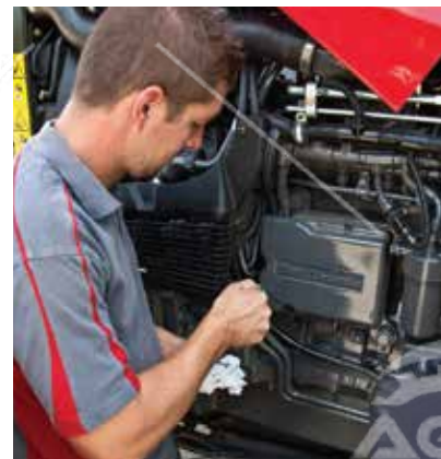
The waisted bonnet and front axle design ensures comfortable access to the engine oil filters and oil dipstick
